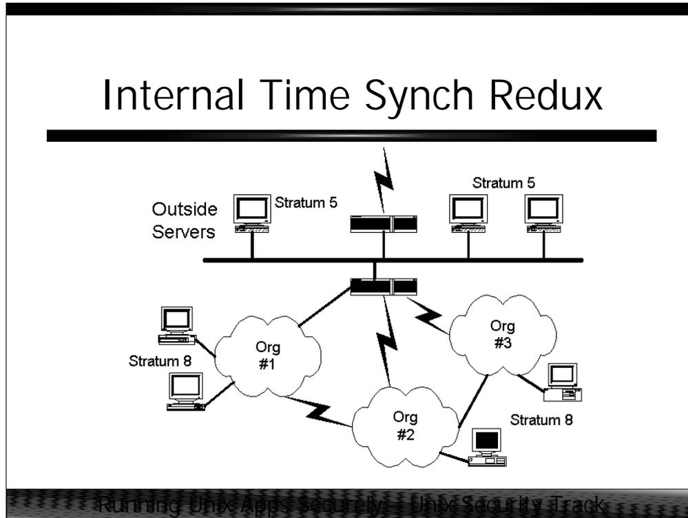
Here's our internal network architecture diagram again, this time showing appropriate stratum values for the various internal and external pseudo-clocks. The pseudo-clocks on the "Outside Servers" should be configured at stratum 5– this means that if the Internet connection becomes severed then the "Outside Servers" will become *stratum 6* servers (the stratum of the pseudo-clock *plus one*).
